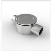
Electrix® Metric Conduit Through Boxes, in 316C16F stainless steel with a 316L - V4A - 1.4404 stainless steel lid, can be used as an inspection point and pull box during a long conduit run.
